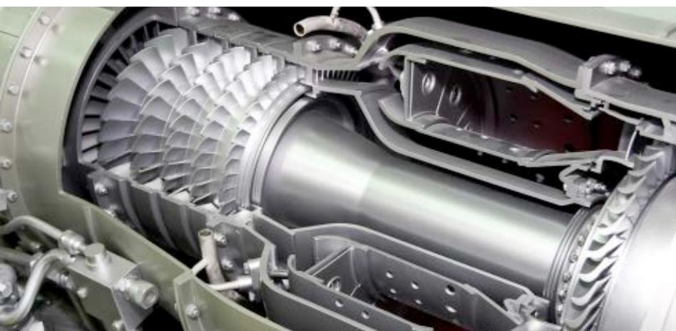
energy technology, and a requirement for keeping those engines in A1 condition. The more weight there is on a rotating turbine blade engine, the higher the centrifugal force, and you want to keep that to a minimum. So a thinner – even incrementally thinner – barrier coating is an advantage, bringing down the weight and reducing the centrifugal force, which in turn reduces wear.
